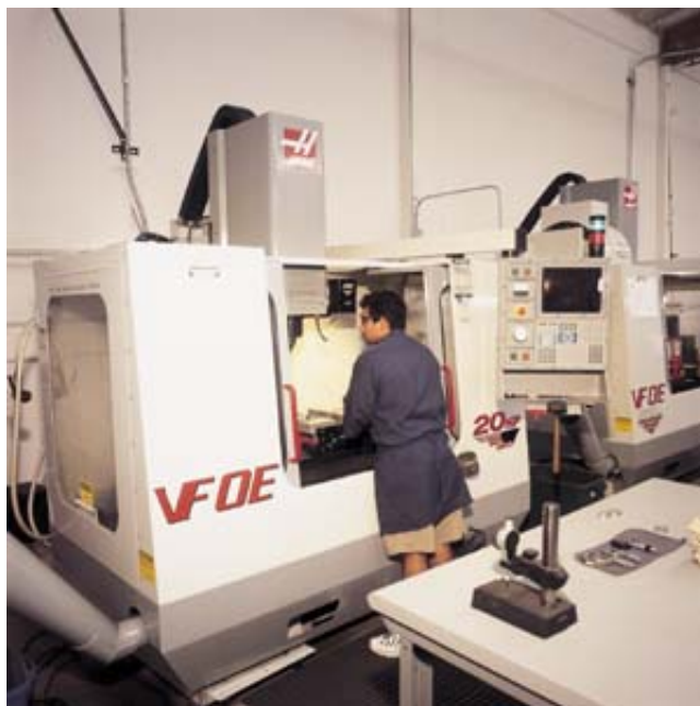
CNC operator, Juan Carlos Heredia, sets up one of Hytron Manufacturing’s HaasVFOE machining centers to produce VIM/VAR components for the modular substrate the company has been licensed recently to produce.
